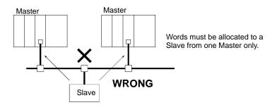
**Note** The master parameter file duplication check from the Configurator can be used to check for node addresses that have been set more than once in the scan list, which shows the I/O allocations that have been made.
